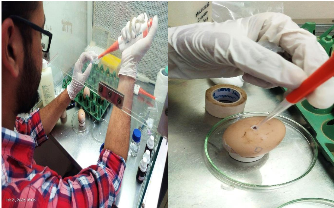
Figure 12 - CAM is inoculated with a sample of the Bellis Perennis drug using a micropipette.
